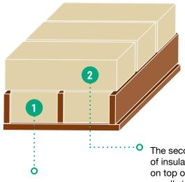
The first layer of insulation is laid between the joists The second layer of insulation is laid on top of the first, usually in a different direction in order to ensure as few gaps as possible
